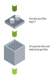
The MG140 is suitable of applications with large volumes of gas and particle filtration, e.g. soldering, adhesives, cleanroom work.
