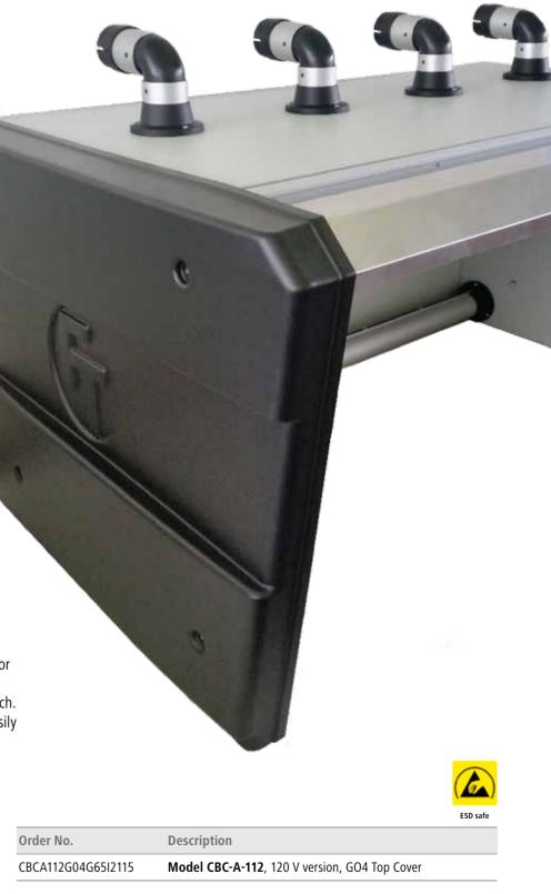
The air curtain cabinet CBC-A has a unique ventilation concept that separates the operator from the process by a dual air curtain system, giving unlimited accessibility on the workbench. It stands directly on the workbench and is easily connected to a FT mobile filter system or to central ventilation.
